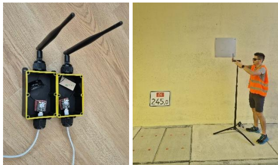
Fig. 2. LoRa communication devices based on the XIAO ESP32S3 and Wio-SX1262 platform used during the tunnel experiments and their placement near the tunnel wall.
