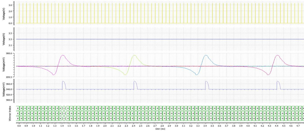
Fig. 3. Device response to pseudo-real particle flow. Behavior of ED logic from a simulated 8×1 GMR-based cytometry array.
