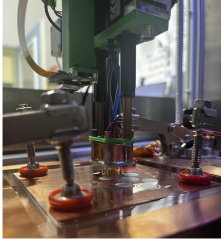
Fig. 4. Interior view of the automated measurement system. The spring-loaded pogo-pin probe head (centre) is positioned over the silver ink electrode pads on the glass sample. The three-terminal guarded probe configuration is connected to the Keysight B2985A electrometer. The XY gantry allows automated positioning across the sample surface.
