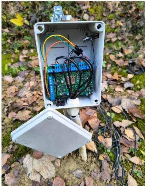
Fig. 1. Prototype of the battery-powered ESP32-C6 sensor node installed in the outdoor environment.
