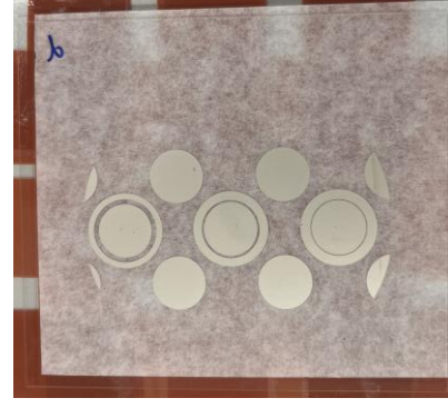
Fig. 2. SCHOTT AS87 eco aluminosilicate glass sample (100 \mu\text{m} ) with tampon-printed silver conductive ink guard ring electrode sets. The three functional patterns correspond to guard gap configurations of 0.1, 0.5 and 1.0 mm and are visible as concentric disk-and-ring structures. Additional ink shapes visible in the image are artefacts of the tampon printing pattern and carry no electrical function.
